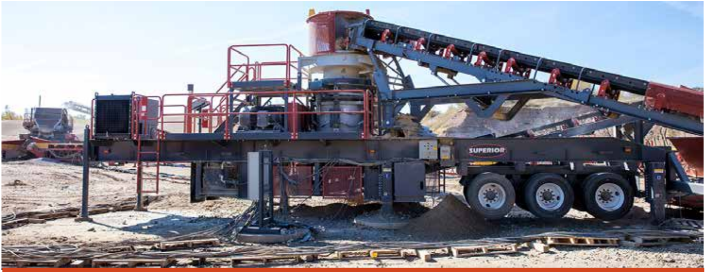
[Figure 1] Cone crusher in plant.
