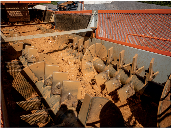
ABRASION-RESISTANT A-532 WEAR PADDLES
